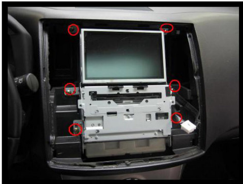
2. Unscrew the bolt and pull the monitor forward. After that, disconnect the connector on back of the LCD.
