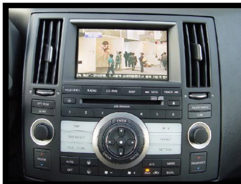
2. Unscrew the bolt and pull the monitor forward. After that, disconnect the connector on back of the LCD.
