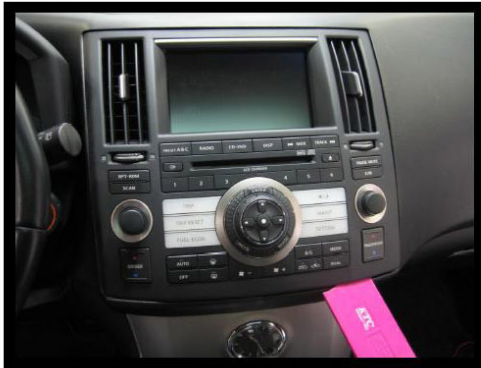
1. Remove the lower part using tool and pull the cover forward to remove it. Don't pull it so hard because there is RIBON CABLE.
