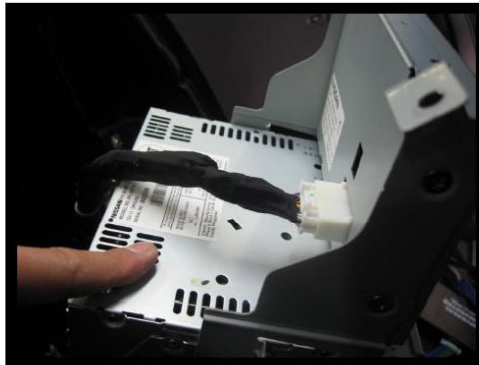
2. Unscrew the bolt and pull the monitor forward. After that, disconnect the connector on back of the LCD.
