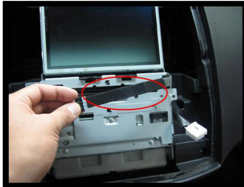
1. Remove the lower part using tool and pull the cover forward to remove it. Don't pull it so hard because there is RIBON CABLE.
